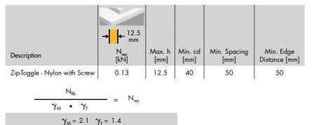
Recommended loads are based on the simplified design method according to ETAG 001, Annex C and are valid for one anchor. For Design loads multiply by the factor  $\gamma_{\rm F}.$
